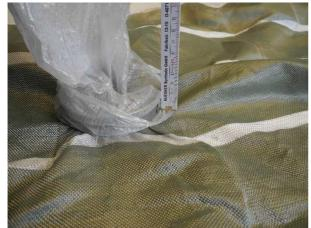
Illustration 11: Double check if the hose clip is completely seated in the groove
