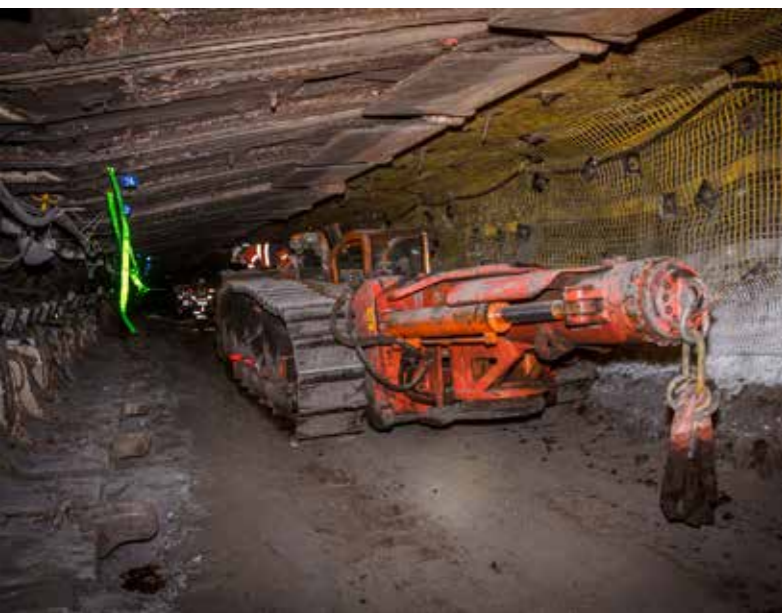
Powered Roof Supports (PRS) in Final position with Dozer preparing to safely remove PRS from face.
