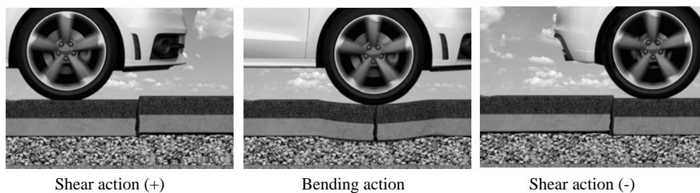
Figure 1. Critical loading cases in a pavement crack
