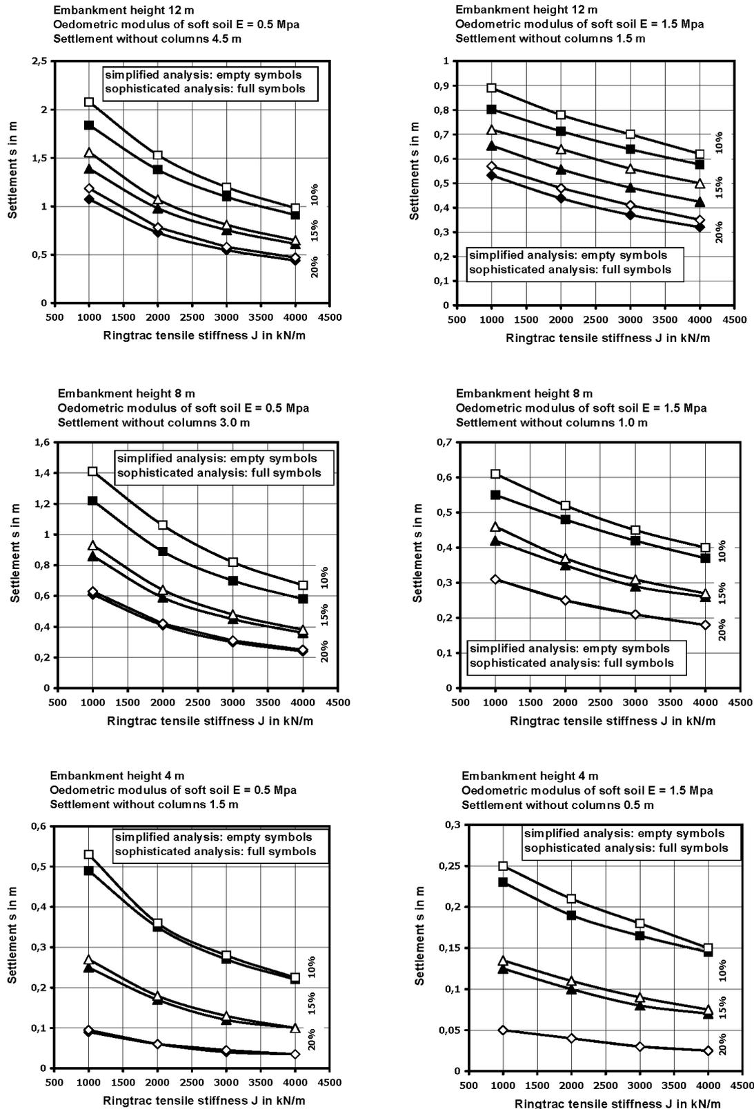
Figure 6. Typical graphs for the settlement depending on the surcharge, the oedometer module of the soft soil, the applied design procedure, the tensile stiffness of Ringtrac<sup>®</sup> and the „percentage
