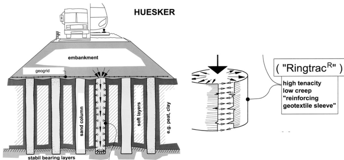
Figure 1. General principle of embankment on soft soil set on geosynthetic-encased columns (GEC)
