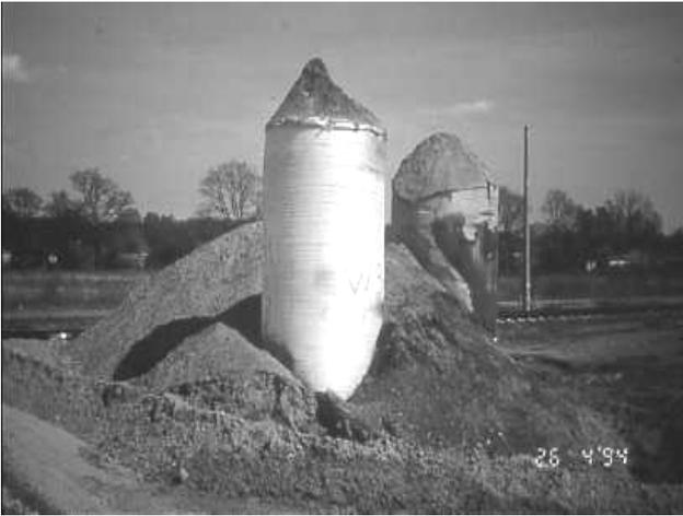
Figure 4. A test column constructed “in air” for a demonstration in a testfield
