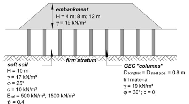
Figure 5. Overview of system analyzed in the examples (graphs)
