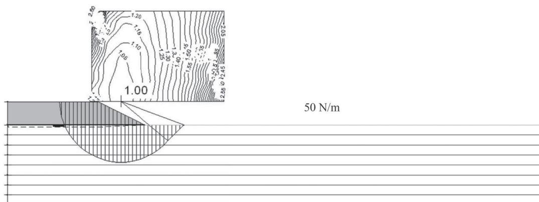
**Figure 11** - Limit equilibrium stability analysis for factor of safety 1.0, allowing to estimate the required reinforcement force,  $T_m$  (*GGU Stability*).
