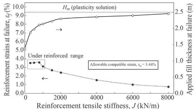
**Figure 9** - Effect of varying  $J$  from 300 to 8000 kN/m on the mobilized reinforcement strains at failure (closed circles, see left-hand side scale) and applied fill thicknesses at failure (open circles, see right-hand side scale) obtained by finite elements simulation of the case study.
