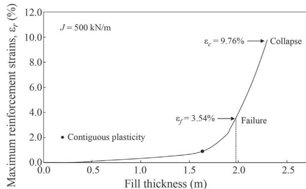
**Figure 6** - Mobilized maximum reinforcement strains during embankment construction obtained by finite elements simulation of the case study with  $J = 500$  kN/m.
