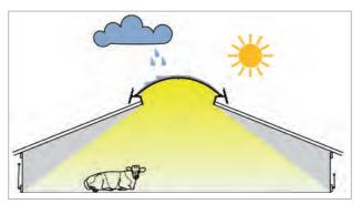
Daylight diffused widely across housing interior by SKYTEX<sup>®</sup> light ridge
